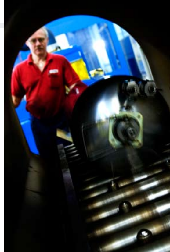
The seals on all stainless steel electric water-heaters are tested in a vacuum chamber.
