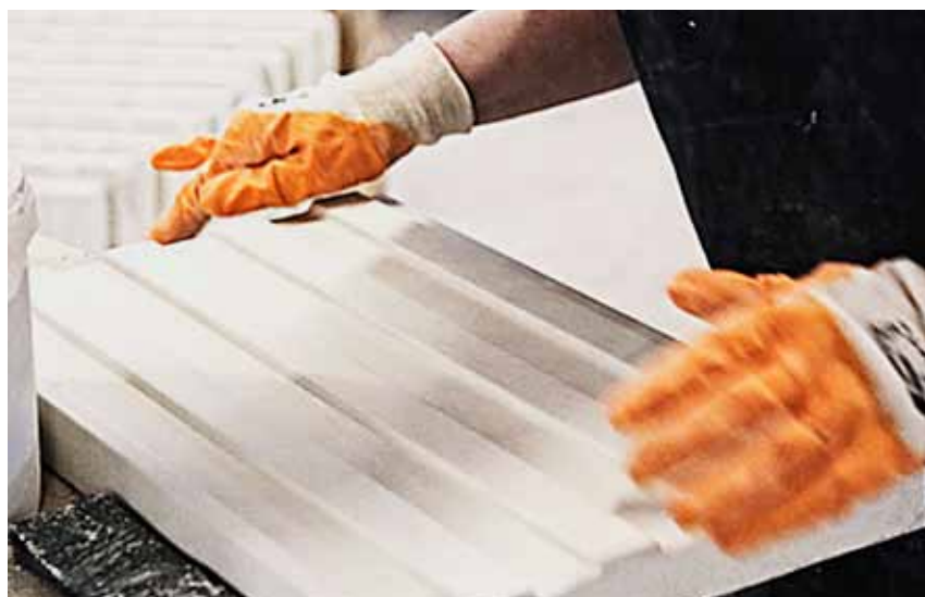
The manufacture of Thermotte, which is used to line fire-boxes, is a precision job that requires skill and a practised, professional hand.
